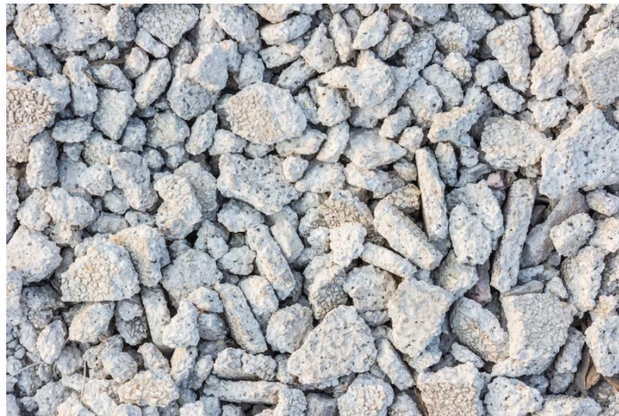
Figure 1 Demolished Aggregates Used in Study
